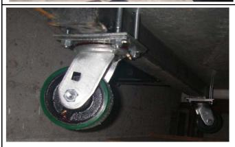
Backing up steep driveway was solved by adding swivel casters to the trailmanor bike hitch receiver. I know longer have to worry about having enough tension in the chains so that the front of the trailer does not jam on the concrete. All is fine now and I no longer have problems with the swing hitch, conflict from the spring bars and the swing hitch post and having the snap brackets break off. This is a bit extreme but is the final solution for me such I don't have to worry about it anymore!!
