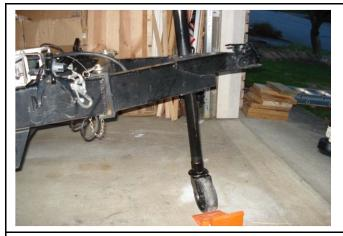
As tension in chains increases backing up steep driveway the bottom of the right side pin pushes against the relatively thin 1/4 inch plate causing it to bend out about 3/4 inch and creating a gap at the bottom of the swing hitch which was a concern for future failure.
