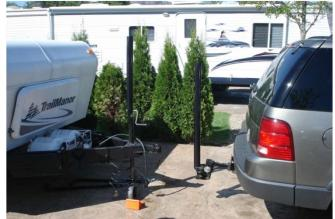
Permanent solution was to get rid of swing hitch and have plates welded to the frame. It will never fail again!
