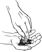
5. Before reinstalling, apply a light coat of grease on the bearing cup.
