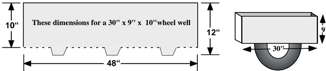
The following procedure can be accomplished with or without removing the trailer tire and wheel. For more working space and more precise placement of the rivets or screws, you may wish to remove the wheel and tire.
