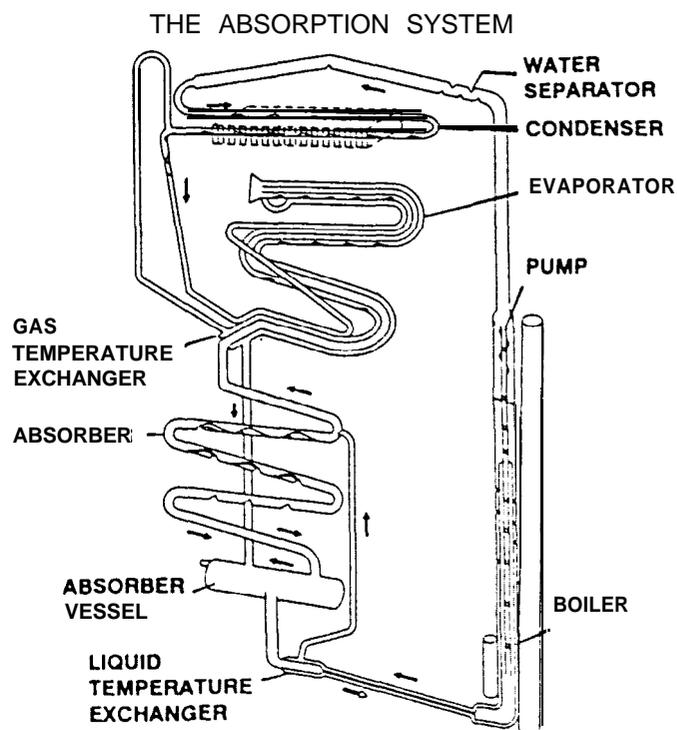
The cooling unit parts<sup>(4)</sup> that accomplish this 'cooling' or heat extraction process, include the:
