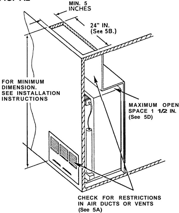
C. Some smaller models may be installed with two side wall vents instead of using a roof vent. For this type of installation make sure the top of the upper vent is the correct distance above the refrigerator. See FIG. A3. The minimum dimension for this measurement is listed in the Installation Instructions for each model.
