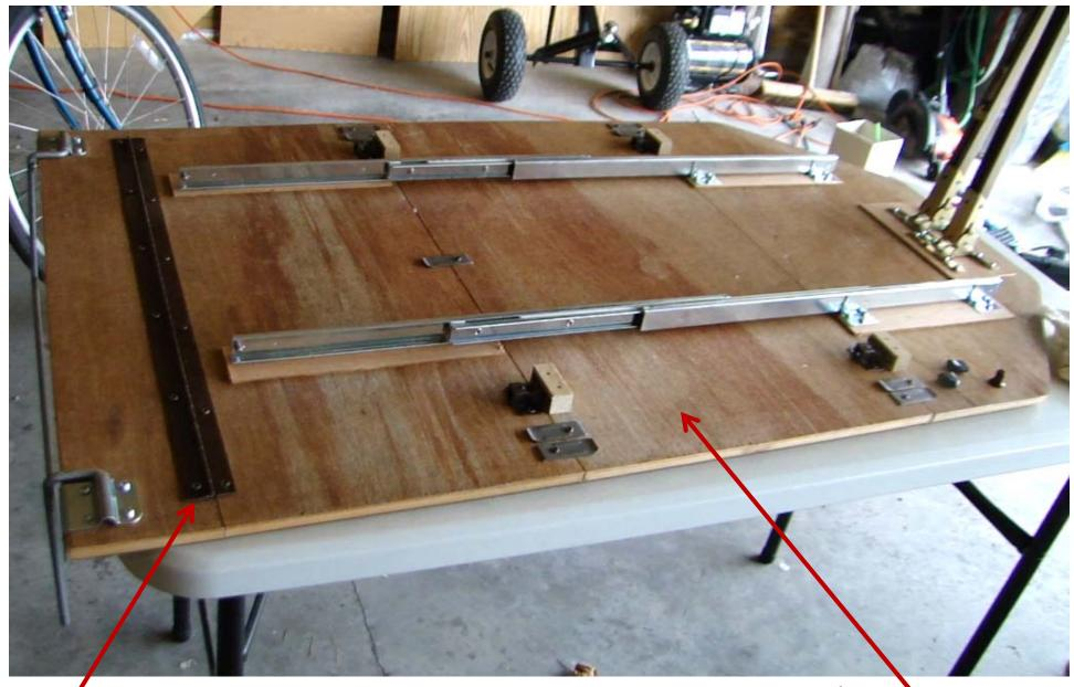
This is the folding part that attaches to the TM wall. I just removed the screws from the piano hinge closest to the main table section, thus allowing me to remove the 4" folding piece. I stored it for future if I ever need it
