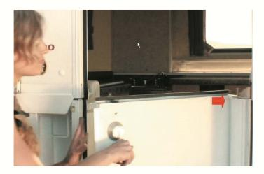
**Step 10:** Open bottom door section, and push outward until pin in the right door frame latches to trailer.
