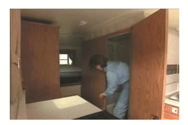
**Step 16:** Swing side bath wall open and latch into place. Note: Raising the rear bath wall closes a switch that energizes the rear roof lights and LP detector. Seal Velcro flaps on roof sections to complete setup.
