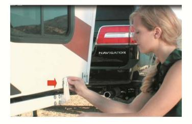
**Step 1:** Release the four white draw latches, one at each corner of the trailer.
