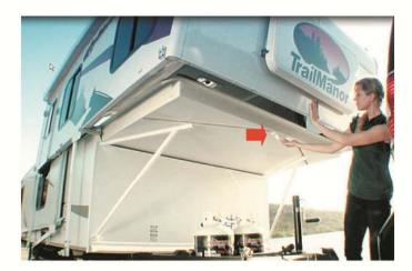
**Step 4:** Using the bed handle, pull out the bed until it stops.
