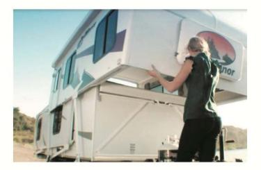
**Step 3:** Standing near the tongue, grasp the lower edge of the front roof section. Lift the front roof up and out in a circular motion beginning with a straight-up motion and finishing with a pull. **Do not lift the roof by the front window stoneguard**. **Do not lift by the sides (risk of pinched fingers).**
