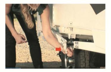
**Step 2:** Release the four black hold down latches, two on each side near the wheels.
