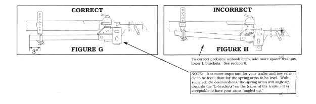
If springs are not approximately horizontal when even settling has been achieved (see Figures G & H), it will be necessary to change the hitch head angle by adding or subtracting spacer washers between the hitch and the shank. L brackets may require readjusting after hitch head angle has been changed.
