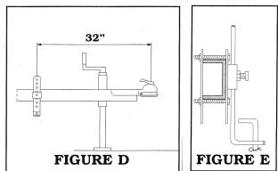
Alternatively, tighten the ½" nuts evenly so that the outside link plate and inside link plate have even contact with the frame before tightening the nuts on the bolts.
