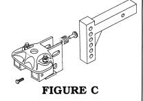
Insert the <sup>3</sup>/<sub>4</sub>" x 4" bolts through <sup>3</sup>/<sub>4</sub>" flat washer hole in the hitch head channel and shank. Install <sup>3</sup>/<sub>4</sub>" flat washer, lock washer and nut. DO NOT TIGHTEN <sup>3</sup>/<sub>4</sub>" BOLTS AT THIS TIME.
