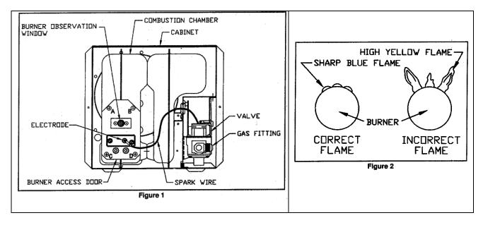
If excessive rust & corrosion are present on the burner surface, the burner must be thoroughly cleaned or replaced. The burner may be cleaned using a steel brush and blown clean using high compression air.
