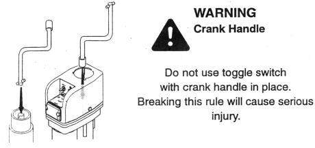
• If the power-head is removed, the crank can still be used to raise/lower the jack. CAUTION: If the power-head is removed, it must be re-synchronized with the jack position.
