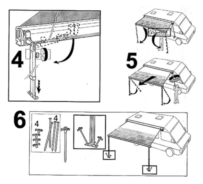
□ **Figure 7** – The support legs can also be fitted to the wall brackets.
