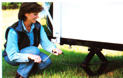
Standard Scissor Jacks Four standard scissor jacks make leveling simple and fast.
