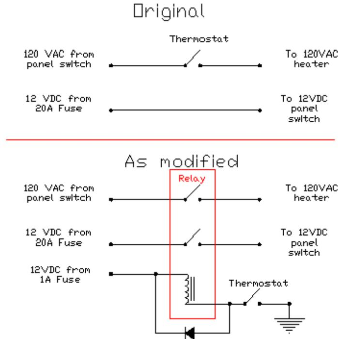
I mounted the relay to the top of the refrigerator using two screws. I put it to the left of the terminal block where the AC and DC power come in. I typed up a schematic and instructions on how to restore the refrigerator to its original configuration, and taped this near the relay. This might minimize the amount of grief I cause future technicians.
